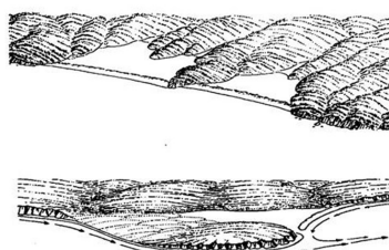
FIGURE 3-10 Upper: Coastal lakes formed by enclosure of lagoons by wave and current-bulk bars on a shore line embayed by slight subsidence. Lower: A land-bounded island with a bay behind it, closed by a sand-reef beach formed by reverse ridge currents. (After Davis, W. M., Coastal J. Marine Geol. , 20-77, 1933.)
